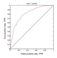
$$\begin{array}{c|cccc} & P & N \\ \hline P^* & TP & FP \\ N^* & FN & TN \end{array} \qquad \begin{array}{c} TPR = TP/P = TP/(TP+FN) \\ FPR = FP/N = FP/(FP+TN) \end{array}$$
